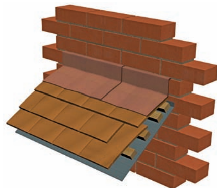
Figure 08: flashing to a top abutment – tiles and slates
