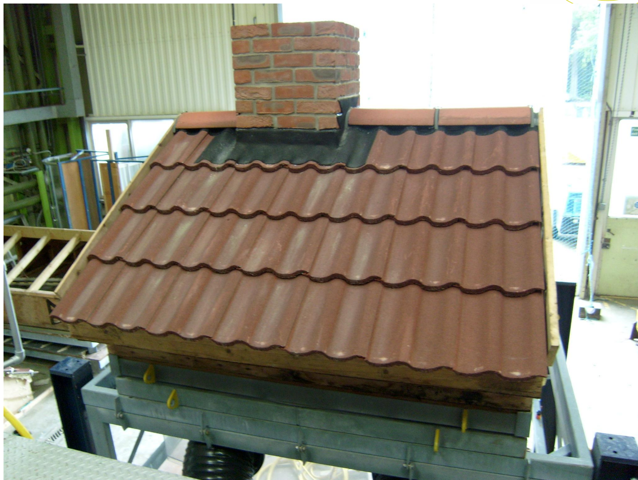
Figure 1. Side 1 Double pantiles and Ubiflex flashing around the chimney.
